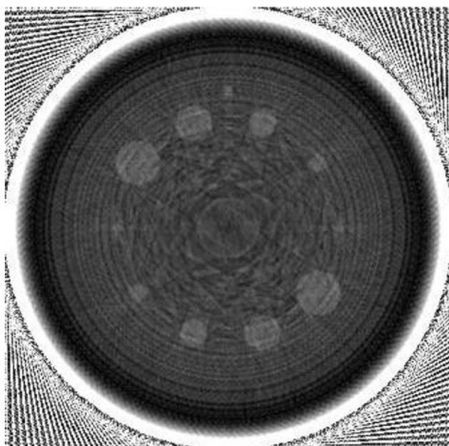
**Fig. 3** The subtracted image from the cone beam reconstruction obtained at 50 keV and that at 25 keV. The weevil is the clearest
