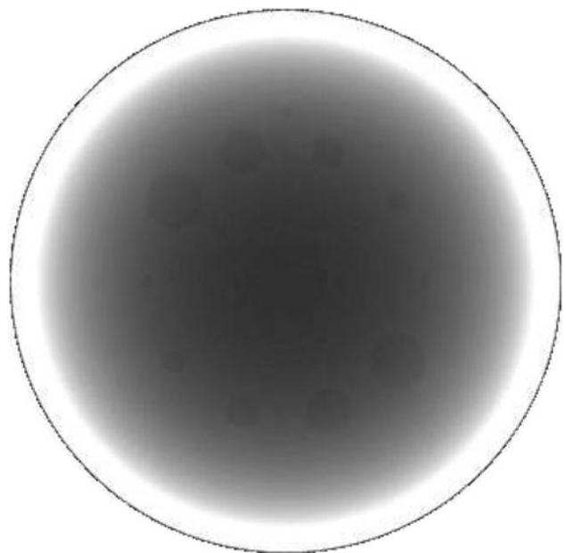
**Fig. 2** A reconstructed cross section of the palm tree model at 50 keV. The weevil becomes much clearer than in a projection image
